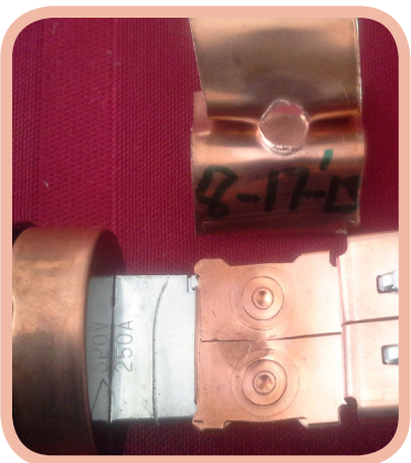
Very low impedance FMRW™ weld of 250 ampere fuse with connector.
