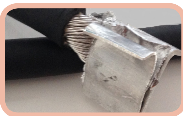
Aluminium cable weld peel tested
