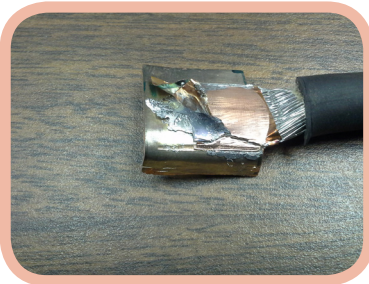
Stranded-wire aluminum cable welded to a copper terminal through an interlayer
